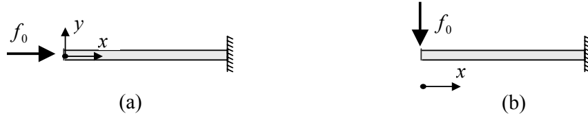
Figure 6. Clamped-free beam given a harmonic force excitation at the free edge. (a) Under longitudinal (x) excitation; (b) under flexural (y) excitation.
