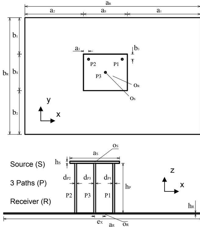
Figure 1. Example case with three parallel paths. Dimensions (all in mm) are as follows:  $a_s = 152.4$ ,  $a_r = 609.6$ ,  $a_1 = 254.0$ ,  $a_2 = 203.2$ ,  $a_3 = 17.8$ ,  $b_s = 127.0$ ,  $b_r = 406.4$ ,  $b_1 = 127.0$ ,  $b_2 = 152.4$ ,  $b_3 = 17.8$ ,  $d_{p1} = d_{p2} = d_{p3} = 6.350$ ,  $e_x = 25.4$ ,  $e_y = 12.7$ ,  $h_s = 6.350$ ,  $h_p = 152.4$ ,  $h_r = 3.175$ . Key:  $O_s$ , center of mass of the source plate;  $O_r$ , center of mass of the receiver plate.
