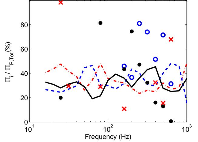
Figure 11. Dissipated power ratio of each path to the total of paths with  $d$  DOF formulation (on one third octave band basis). Key: - - - , path 1 ( $d = 6$ ); - - - , path 2 ( $d = 6$ ); —, path 3 ( $d = 6$ ); X, path 1 ( $d = 1$ ; Z); O, path 2 ( $d = 1$ ; Z); •, path 3 ( $d = 1$ ; Z). Only values between 0 and 100 % are shown for 1DOF formulation.
