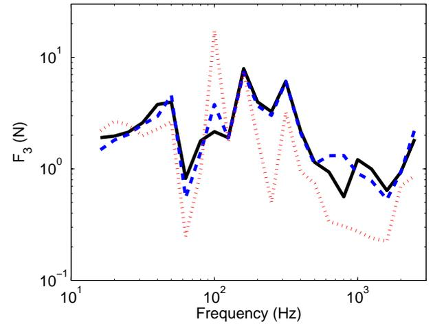
Figure 9. Interfacial path force magnitude spectra at the junction of source and path 3 (on one third octave band basis). Key: —, direct and indirect 6DOF formulations; - - - , 3DOF (X, Y, Z) formulation; · · · · , 1DOF (Z) formulation.
