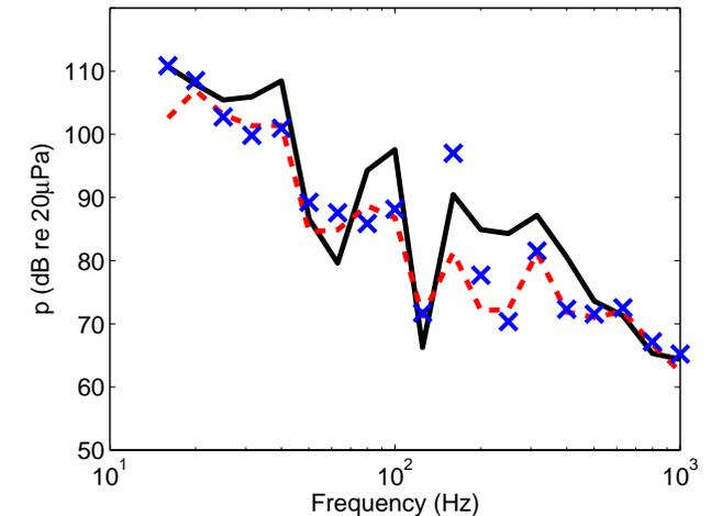
Figure 7. Sound pressure (total) magnitude on one third octave band basis. Key:  $\text{—}$ , direct estimation;  $\text{- - -}$ , 6DOF formulation; X, 1DOF (Z) formulation.
