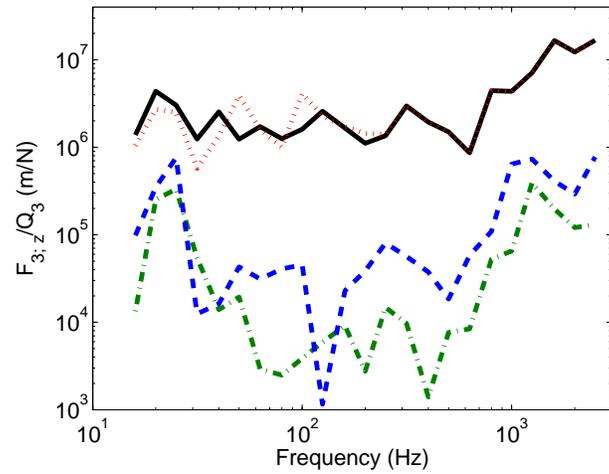
Figure 5. Dynamic stiffness (on one third octave band basis) with respect to  $F_{3;z}$  for the path-receiver subsystem estimated by inverting the compliance matrix.
