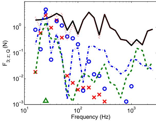
Figure 4. Partial force of  $F_{3;z}$  magnitude spectra (on one third octave band basis). The 3-path sum as given by Equation (4); key: —,  $F_{3;z}$  (total); X, x-term; O, y-term; ····, z-term; - - - ,  $\psi$ -term; - - - ,  $\theta$ -term;  $\Delta$ ,  $\phi$ -term.
