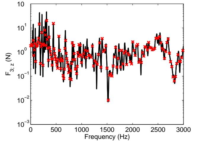
Figure 3. Interfacial force magnitude spectra in the z-direction at the junction of source and path 3 (on narrow band basis). Key: —, direct method by Equation (1); X, indirect method by Equation (2).
