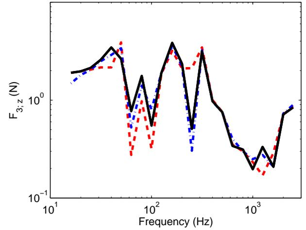
Figure 8. Interfacial path force magnitude spectra in the z-direction at the junction of source and path 3 (on one third octave band basis). Key: —, direct and indirect 6DOF formulations; - - - , 3DOF (Z,  $\Psi$ ,  $\Theta$ ) formulation; - · - · , 3DOF (X, Y, Z) formulation.
