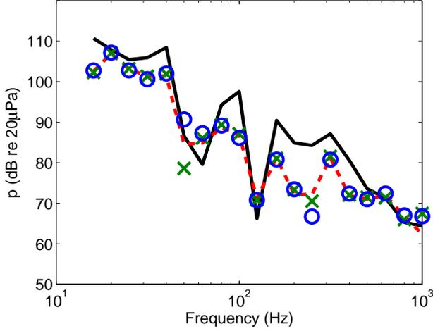
Figure 10. Sound pressure (total) magnitude on one third octave band basis. Key: —, direct estimation; - - - , 6DOF formulation; X, 3DOF (X, Y, Z) formulation; O, 3DOF (Z,  $\Psi$ ,  $\Theta$ ) formulation.
