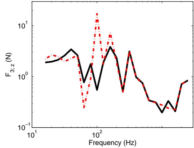
Figure 6. Interfacial path force magnitude spectra in the z-direction at the junction of source and path 3 (on one third octave band basis). Key:  $\text{—}$ , direct and indirect 6DOF formulations;  $\text{- - -}$ , 1DOF (Z) formulation.
