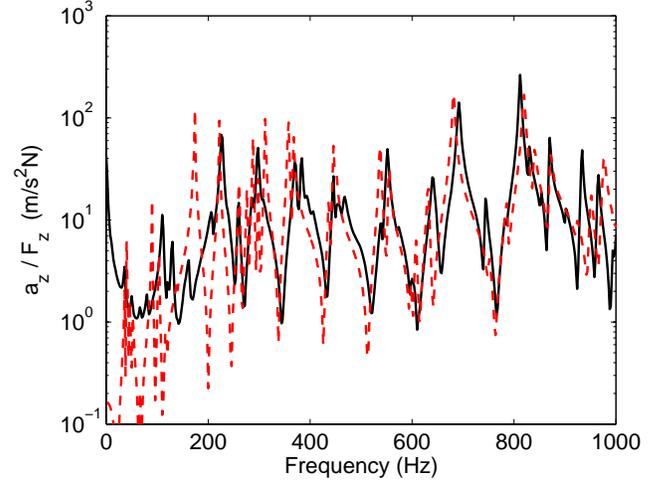
Figure 2. Driving point acceleration of the example case of Figure 1 on narrow band basis. Key: —, experiment; - - -, model.
